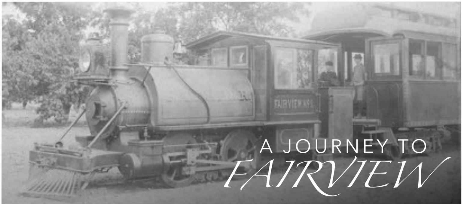
The Fairview No. 1 steam locomotive was a narrow-gauge engine in the 0-4-2T configuration. Photograph by Conaway & Hummel.
